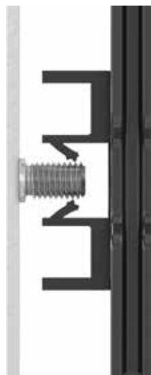
Mounting the rod guide on the welding studs
