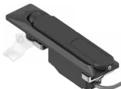
Two countersunk screws M3 included in scope of delivery. Cross recess and hexagon female SW 2 with pin.
