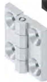
Screw-on hinge for countersunk screw M4; zinc die surface of choice; hinge pin stainless steel
