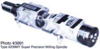
Type 4209MY Super Precision Milling Spindle with Timken 'Hydra-Rib' design bearings. Housing is arranged for recirculating oil cooling and includes linear power drawbar assembly.
