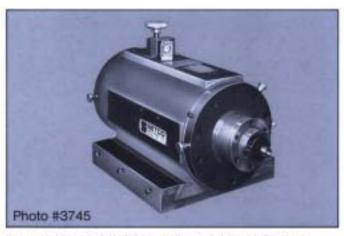
Type 16120-144MLCY High Speed, Liquid Cooled Motorized Milling Spindle rated 20 HP at 14,400 RPM with oil mist lubrication to the bearings, #40 NMTBA nose, shaft lock with electrical safety interlock, manual drawbar and base having a male dovetail.
