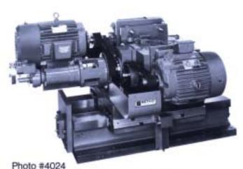
Special Cluster Spindle/Hardened Steel Way Slide Assembly illustrating a rotating hydraulic cylinder package and individual drive packages for each spindle assembly all mounted on a 24" wide slide with internally mounted hydraulic cylinder package.
