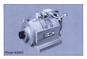
Type 16130-144MLCY High Speed Liquid Cooled Routing Spindle equipped with quick change tool holder, manual shaft lock, standard air purge lines and regulator, coolant inlet-outlet and arrangement for oil mist lubrication to the bearings. The precision spindle is rated 30 HP/14,400 RPM/230 volts to approximately 3.5 HP/1800 RPM/29 volts.
