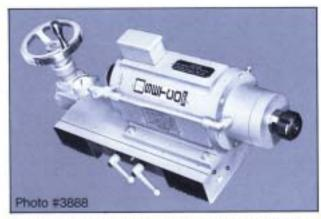
Type 16110-144MLCY Liquid Cooled Routing Spindle with integral collet nose assembly having a collet capacity up to 1" diameter. The spindle is designed to operate from 3600 RPM to 14,400 RPM at 15 HP for machining honeycomb composites and aluminum. These spindles were mounted on 12" centerlines and include a precision ground 10" dovetail slide (ref. Catalog 183) with right angle attachment, bellows and manual gib locks.
