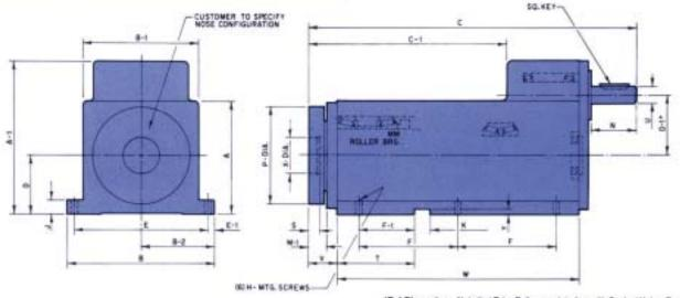
\*D-1 Dimension—Note that Drive Pulley may interfere with Coolant Union, Power Draw Bat, etc. . . .
