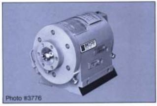
Type 16102-500MLCY Liquid Cooled Routing Spindle rated 2 HP at 50,000 RPM and arranged to operate at a low end of 36,000 RPM. The spindle is arranged with straight shank nose, oil mist lubrication to bearings and dovetail mounting. Spindle used in an aluminum routing operation.
