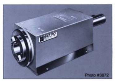
The SETCO 4300M Series of Super Precision Milling Spindles have the same high quality standards as the 4300B Series Boring Spindles shown on page 8. These spindles include a triplex set (except size 4302M) of select fit bearings which are ideal for axial and radial thrust loads experienced during heavy duty metal removal with milling cutters.
