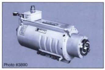
Type 16115-72MLCY Liquid Cooled Milling Spindle arranged to operate infinitely variable from 450 RPM/4.5 HP/30 hertz to 7200 RPM/24 HP/120 hertz (2/8 pole motor winding). Spindle arranged for dynamic braking through the frequency converter, #50 NMTB Nose, manual draw bar, manual shaft lock with electronic safety interlock, oil mist lubrication to the front and rear bearings and oil mist reclassification system.
