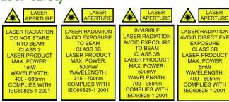
The light emitted from these devices has been set in accordance with IEC60825. However, staring into the beam, whether directly or indirectly, must be avoided. IEC60825 classifies laser products into 3 categories depending on light emitted, wavelength and eye safety.
